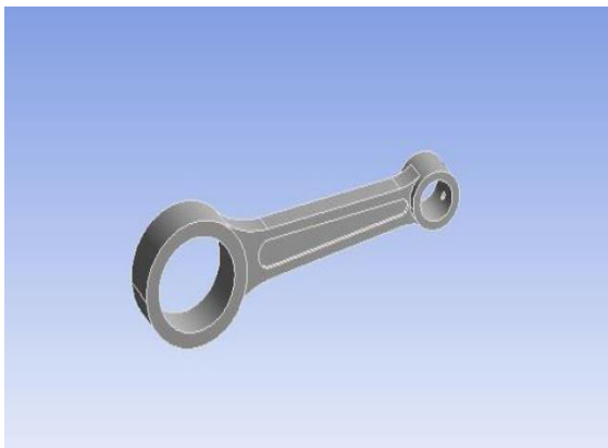
Fig. 2.1 3D Model of Connecting rod in Autodesk fusion 360
